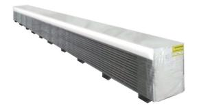
For safe transportation are sandwich panels packed by 18 pieces in stacks long up to 13500 mm. The corners and the sides of the stack are covered in polystyrene and the whole package is wrapped in foil.
